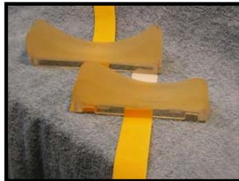
Figure 4. Standoff pads with Velcro
