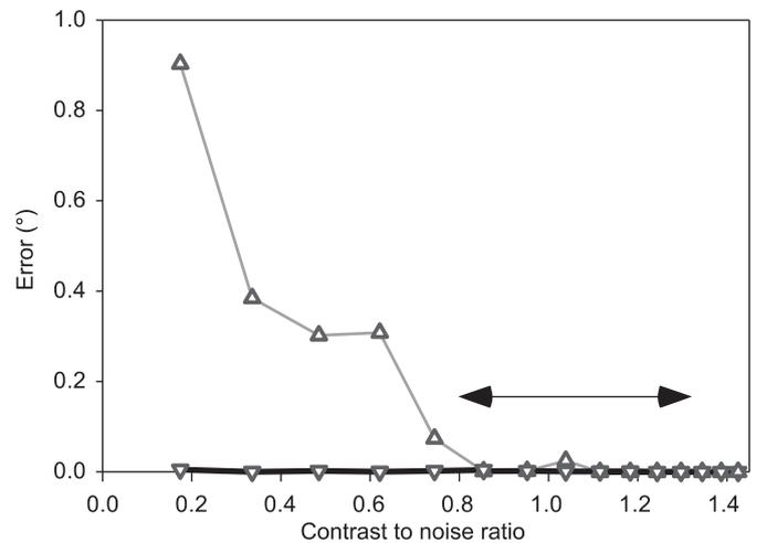
**Fig. 8.** Errors in the estimated orientations from the simulated grids calculated for a range of contrast to noise ratios at a fixed orientation of  $8.6^\circ$ . Angles calculated using the wavelet transform are shown by the grey line and triangles with apex at top, and angles calculated using the Radon transform are shown by the black line and triangles with apex at their bottom. The arrows show the range of contrast to noise ratios observed in ultrasound images from the vastus lateralis.
