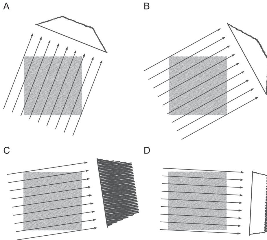
**Fig. 4.** An illustration of the Radon transform at four different angles  $\theta$  on a synthetic grid (A–D). The arrows show the projections through the grid. The Radon transform shows the greatest variance when  $\theta$  approaches the orientation within the grid.
