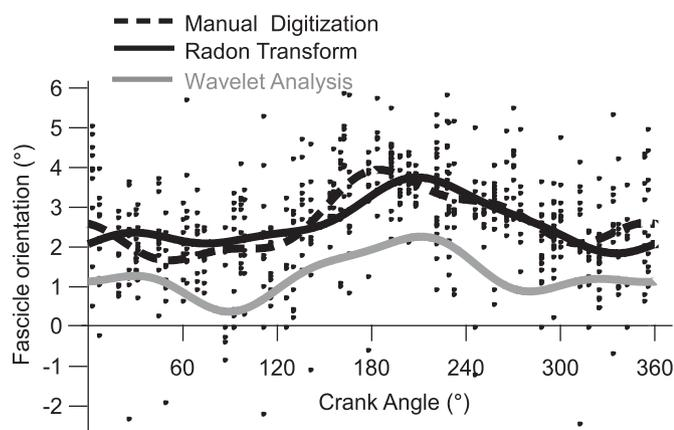
**Fig. 9.** Muscle fascicle orientations in the vastus lateralis during cycling. Orientations are relative to the ultrasound probe (skin) surface. Points show the orientations determined from manual digitization by 10 researchers. Lines show the orientations determined using Fourier series from the manually digitized points (dashed black line); Radon transform (solid black line) and wavelet transform (solid grey line).
