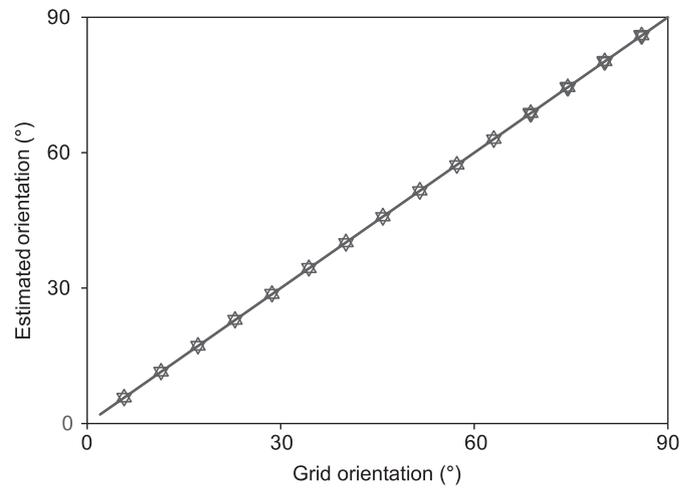
**Fig. 7.** Estimated orientations from the simulated grids calculated for a range of angles using  $\text{CNR} = 0.75$ . Angles calculated using the wavelet transform are shown by triangles with apex at top, and angles calculated using the Radon transform are shown by triangles with apex at their bottom. The line shows the ideal result.
