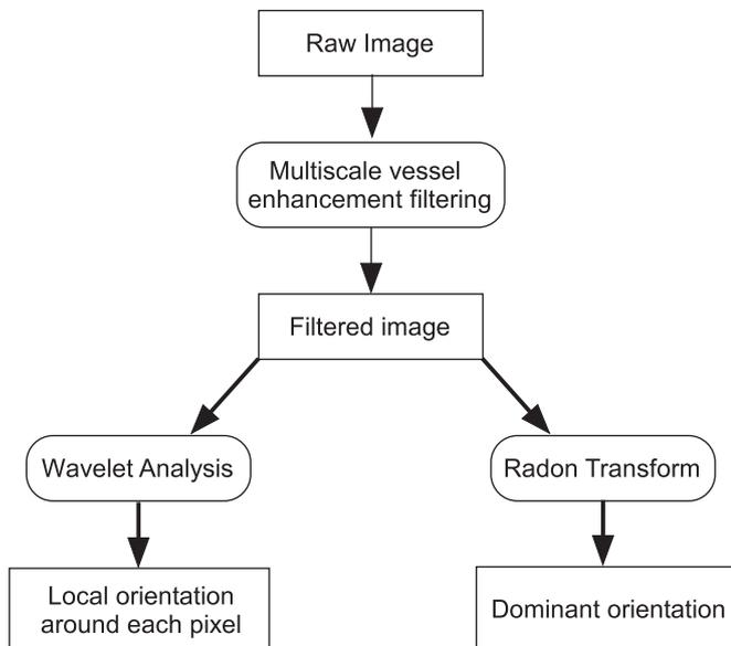
**Fig. 1.** The sequence of methods used to determine fascicle orientation.
