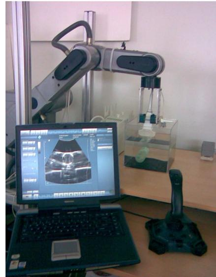
**Figure 3.** The 3D US robotic experimental setup. The robotic arm carries the probe and the position sensing receptor from the US scanner and the spatial locator, respectively. The workstation personal computer controls the movements of the robotic arm with the aid of a joystick. Images are tagged with their spatial location and showed on the screen.
