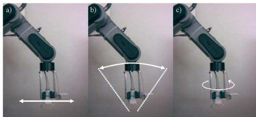
**Figure 2.** Acquisition modes: linear (a), fan-like (b) and rotatory (c) scans.
