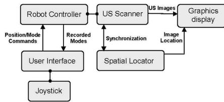
**Figure 1.** Block diagram of the Medical Robot system.
